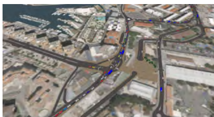
MICROSIMULATION SOFTWARE IS BEING USED TO ASSESS AND TEST A VARIETY OF TRAFFIC MANAGEMENT OPTIONS IN THE CITY CENTRE INCLUDING POSSIBLE PEDESTRIANISATION OF MARKET PLACE.
